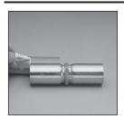
Insertion Depth - Mark hose end with proper insertion depth line.
