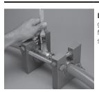
**Lubricate** – Using SAE 20 oil, generously lubricate the steel fitting surface and ID of the swage dies.
